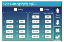
**V(W)**: It is used to adjust the inverter active power according to the set grid voltage.
