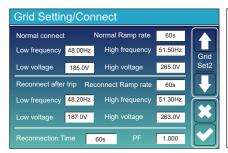
Normal connect: The allowed grid voltage/frequency range when the inverter first time connect to the grid.
