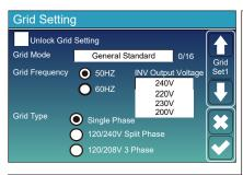
**Unlock Grid Setting:** before changing the grid parameters, please enable this with password. Then it is allowed to change the grid parameters.
