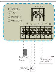
TEMP(1,2): battery temperature sensor for lead acid battery.
