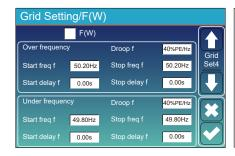
**FW**: this series inverter is able to adjust inverter output power according to grid frequency.
