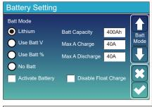
**Battery capacity:** it tells hybrid inverter to know your battery bank size.
