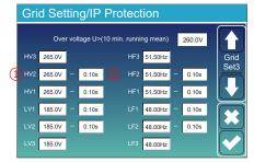
HV1: Level 1 overvoltage protection point;
